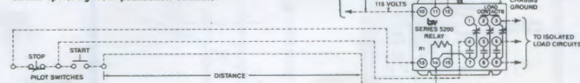
Series 52 solid state relay with built in holding circuit operating from pushbutton contacts.
