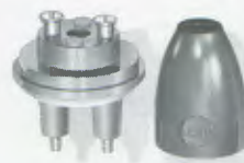
TYPE SE-1—SE-4 HOLDERS Mounting: 2" sanitary fitting. Electrode Studs: \frac{1}{4} —20 male.
