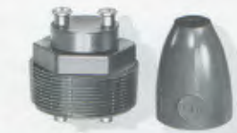
TYPE AE-2 HOLDER Mounting thread: Std. 2" pipe. Electrode Studs: \frac{1}{4} —20 female.
